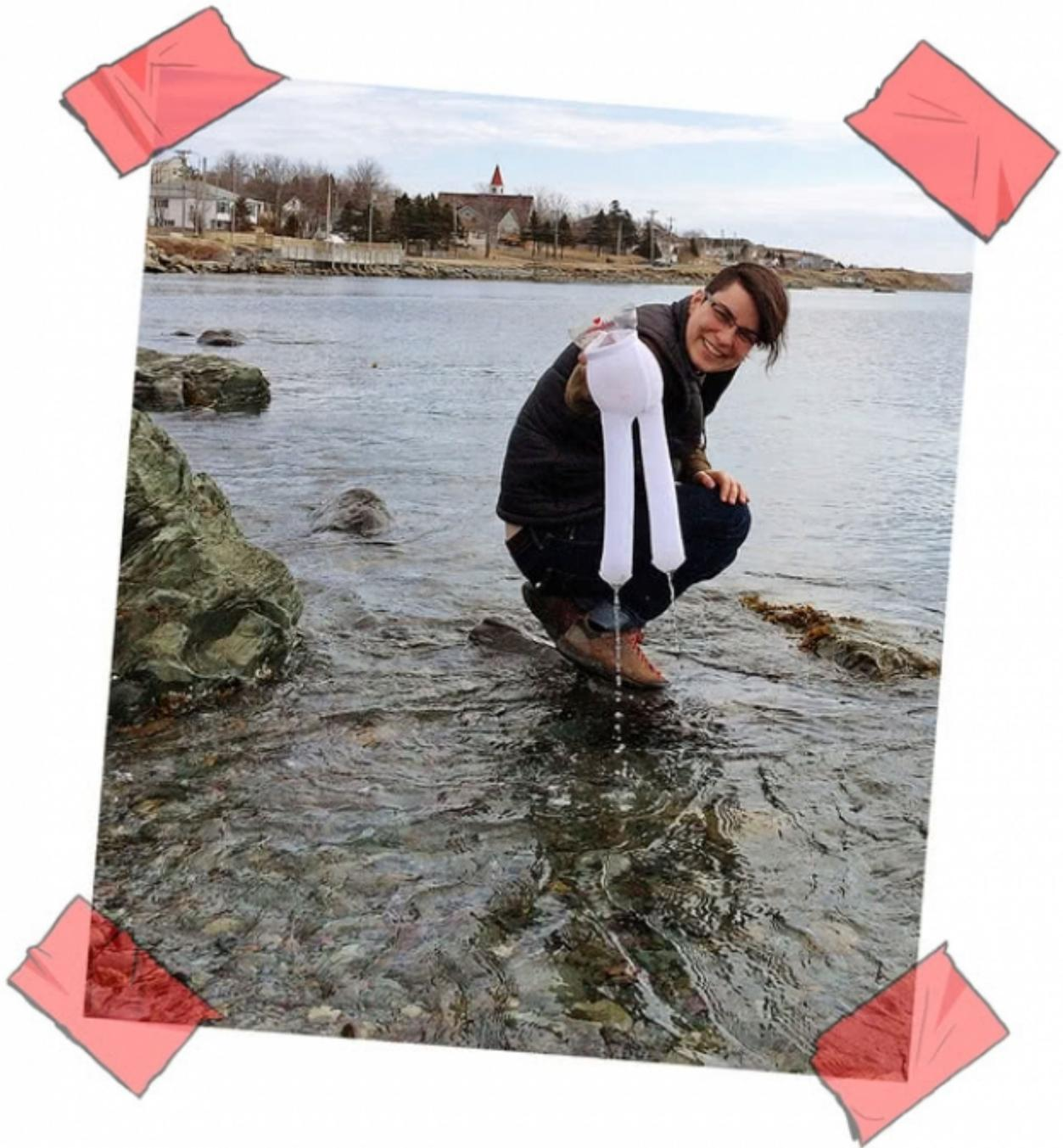
A PAIR of toddler's tights. That is the most important component of the device that Max Liboiron designed to measure the ocean's plastic debris.
